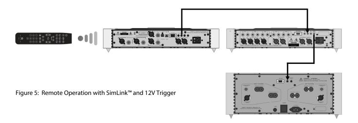
In figure 5 we have a **650D** DAC connected to a **740P** Preamplifier via their respective SimLink™ ports (using a 1/8″ mini-jack cable), and the **740P** is connected to a **870A** Amplifier via their respective 12V triggers (also using a 1/8″ mini-jack cable). When you turn on the **650D** via remote control (or its Standby button), both the **740P** and **870A** will turn on automatically. The same rule applies when you put the **650D** into Standby mode.
