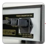
a) Connect the mains cable to the IEC mains input socket.
