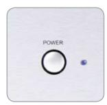
b) Press power switch. The LED power indicator will light up. The pre-amplifier output relay will click after a 6-second delay, together with the indicator lights on the volume knob and one source button.
