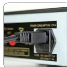
b) Connect the mains cable to the IEC mains input socket.
