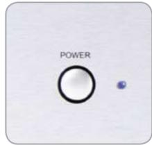
b) Press power switch. The LED power indicator will light up. The pre-amplifier output relay will click after a 6-second delay, together with the indicator lights on the volume knob and one source button.
