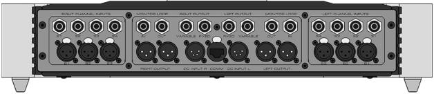
Figure 3: Rear panel of the MOON 850P Preamplifier
