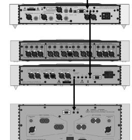
Figure 6: Remote Operation with SimLink™and 12V Trigger
