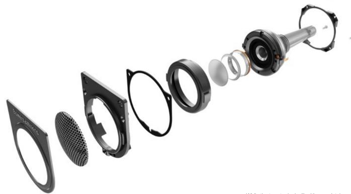
While the tweeter looks like it's completely integrated into the cabinet of each speaker in the 600 Series, it's actually kept physically isolated from the enclosure that surrounds it. The tweeter sits in a ring of gel that acoustically decouples it from its housing, so performance isn't hit by unwanted resonances and vibrations. Imaging and dispersion are improved, delivering a more natural, spacious sound.
