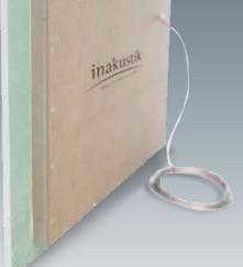
Power: 60 Watt Impedance: 6 Ohm Frequency: 80–18,000 Hz Sensitivity: 92.5 dB Overload Protection (PTC) Dimensions: 625 x 500 x 44 mm (H x W x D) Weight: 5.8 kg approx. System: 2 way Beam Angle: H x V 180° x 180° Connection: 10 m speaker cable, colour coded Max. SPL: 108 dB Support: 12.5 mm gypsum plaster board
