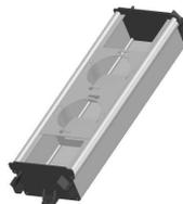
2.) Pull the cables through the end sections and fix them in place with the strain relief (separate item). Screw the end sections to the base section of the accessory box.
