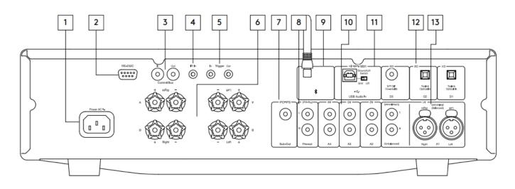
**1. AC power socket** - Once you have completed all connections to the amplifier, plug the AC power cable into an appropriate mains socket then switch on. Your amplifier is now ready for use.
