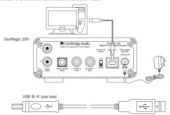
Note: Always use a certified cable for USB Audio, preferably one that displays an official USB Audio 2.0 the cable should be the 'Hi-Speed USB' certified. USB cable connections longer than 3m may result in inconsistent audio performance.
