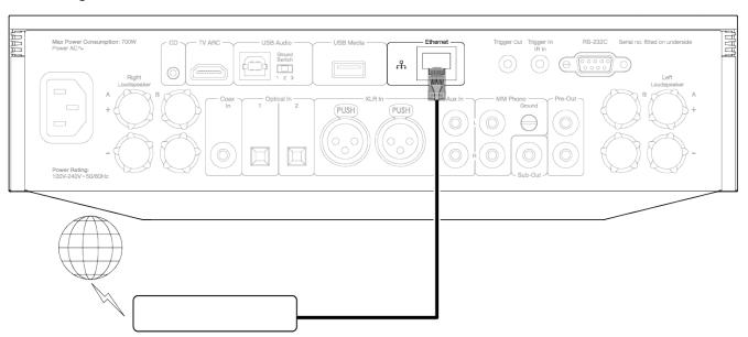
Connect a network cable between the Evo and your router.
