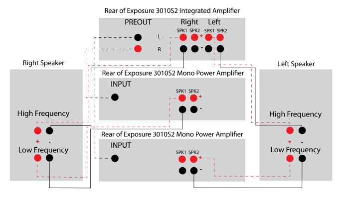
Connecting a pair of loudspeakers in Bi-amping mode
