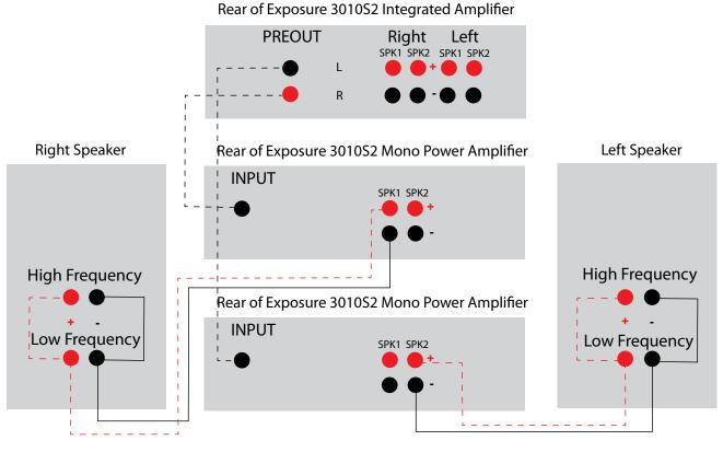
Connecting a pair of loudspeakers using separate Power Amplifiers
