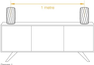
Diagram 1 Stereo positioning
