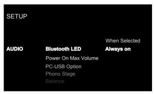
This Audio menu in the Setup menu, provides the following options, selected by placing the highlight on the desired line using the  $^{\wedge}/_{\checkmark}$  D arrow buttons and pressing the Enter K button. This action displays the right side options allowing changes. Change the options using the  $^{\wedge}/_{\checkmark}$  D arrow buttons and press the Enter K button to confirm.
