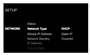
This Network menu in the Setup menu, provides the following options, selected by placing the highlight on the desired line using the  $^{\wedge}/_{\checkmark}$  D arrow buttons and pressing the Enter K button. This action displays the right side options allowing changes. Change the options using the  $^{\wedge}/_{\checkmark}$  D buttons and press the Enter K button to confirm.
