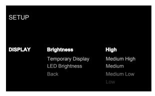
This Display menu in the Setup menu, provides the following options, selected by placing the highlight on the desired line using the ^/ $\checkmark$  D arrow buttons and pressing the Enter k button. This action displays the right side options allowing changes. Change the options using the ^/ $\checkmark$  D arrow buttons and press the Enter k button to confirm.
