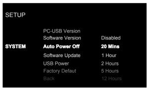
This System menu in the Setup menu, provides the following options, selected by placing the highlight on the desired line using the  $^{\wedge}/_{\bigcirc}$ 0 arrow buttons and pressing the Enter  $^{\textcircled{k}}$  button. This action displays the right side options allowing changes. Change the options using the  $^{\wedge}/_{\bigcirc}$ 0 arrow buttons and press the Enter  $^{\textcircled{k}}$  button to confirm.
