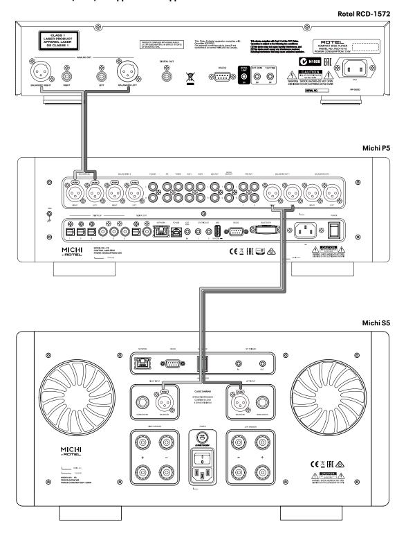
Figure 5: Digital Inputs and 12V Trigger Output
