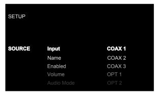
A key step in setting up the unit, is to configure each source input using the Source Setup screens. Configuring the inputs allows you to set defaults for a number of settings including the type of input connector, the desired audio mode, custom labels that appear in the displays when a source is selected, and many more options.
