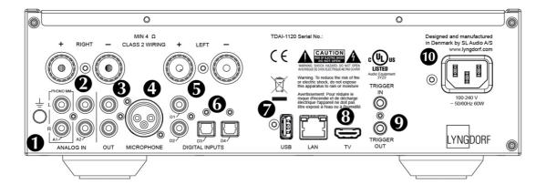
**1. A1/PHONO MM:** Connects directly to turntables/gramophones with high output cartridges (MM: Moving Magnet). The ground cable from the turntable/gramophone connects to the finger screw.
